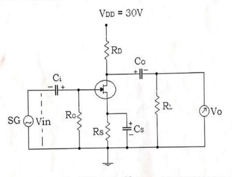
FET- BF245C $R_G = 1 \ M\Omega$  $Ci = 2 \ D\mu F$ SG - signal generatorRd = 10 K\Omega $R_L = 2 \ DK\Omega$  $Co = 2 \ D\mu F$ Vo - AC millivoltmeterRs = 3 & SONVDD = 30 VCs =  $D \ D\mu F$
